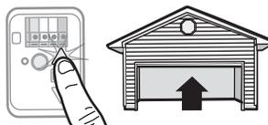
**NOTE:** The UP and DOWN Buttons can be used to move the door up and down as needed.
