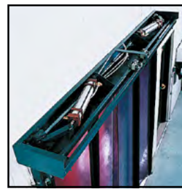
Pneumatic cylinders in door head (non-stainless steel model shown)
